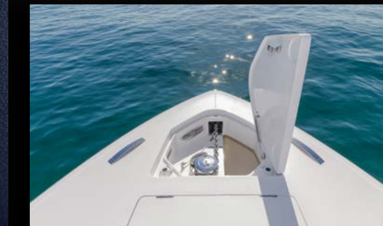
► A hideaway windlass with a large bow storage area just behind it.
